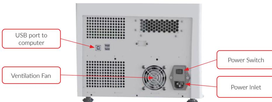
**Figure 2.3** The back panel of the M220 instrument
