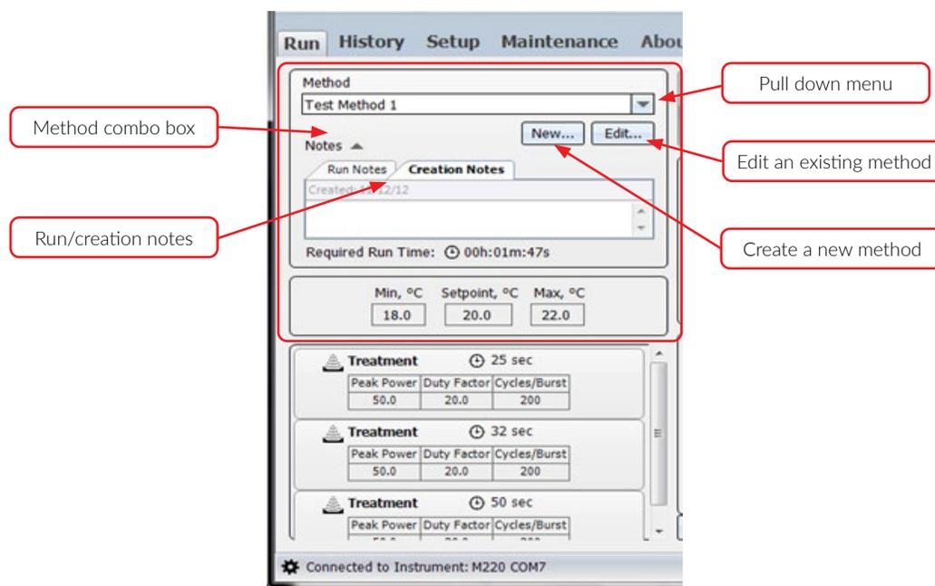
Figure 3.2 Selecting and loading an acoustic method
