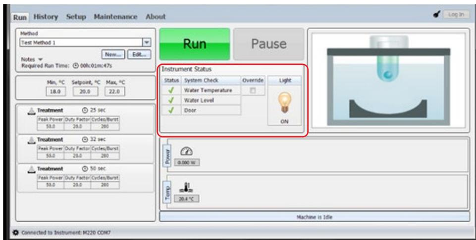
Figure 3.3 Instrument Status Panel and Instrument Light Control
