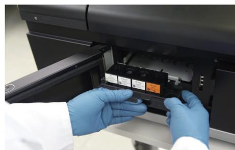
**Fig 2.** Users can easily exchange the filters in Amersham Typhoon 5 and RGB models. If a new filter is inserted or a filter is changed, the instrument automatically recognizes the filter and updates the control software.
