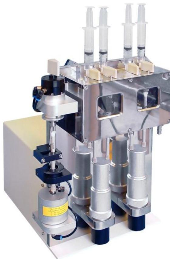
Figure 2.35: sequential-mixing SHU in sequential-mixing configuration
