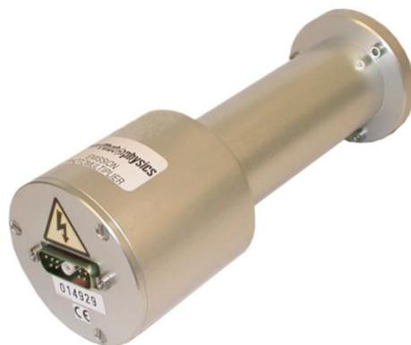
Figure 3.23: the standard fluorescence detector
