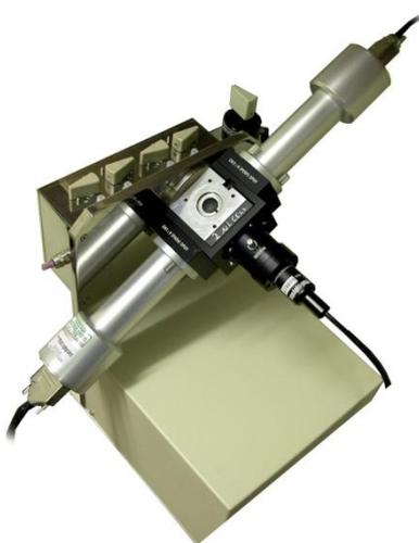
Figure 2.20: the fluorescence polarisation accessory
