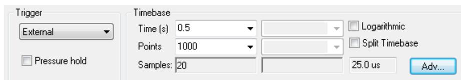
Figure 2.10: the Trigger and Timebase panels for absorbance kinetics
