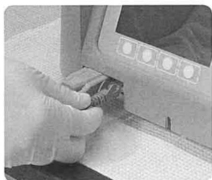
Fig. 16. Ethernet connection.
