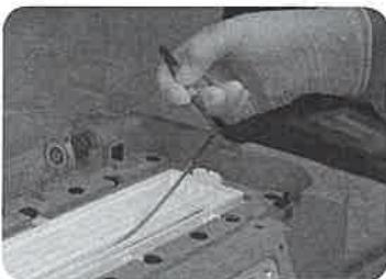
**Fig. 19.** Load the IPG strips.
