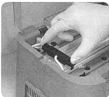
**Fig. 24.** Lock (+) electrode in place.
