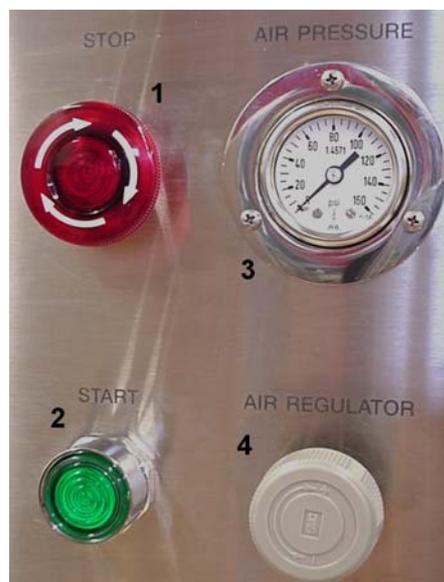
**Figure 2:** Close up view of the standard controls on the EmulsiFlex-C3 control box.
