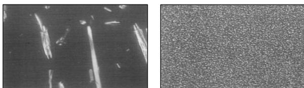
**Figure 12:** Unprocessed dispersion (10-100microns, left) and processed, uniform dispersion (1micron, right) using an EmulsiFlex homogenizer at 25000psi/173MPa.
