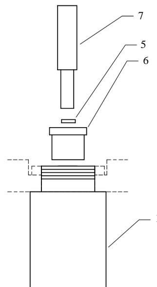
**Figure 9:** EmulsiFlex-C3 plunger seal insertion.
