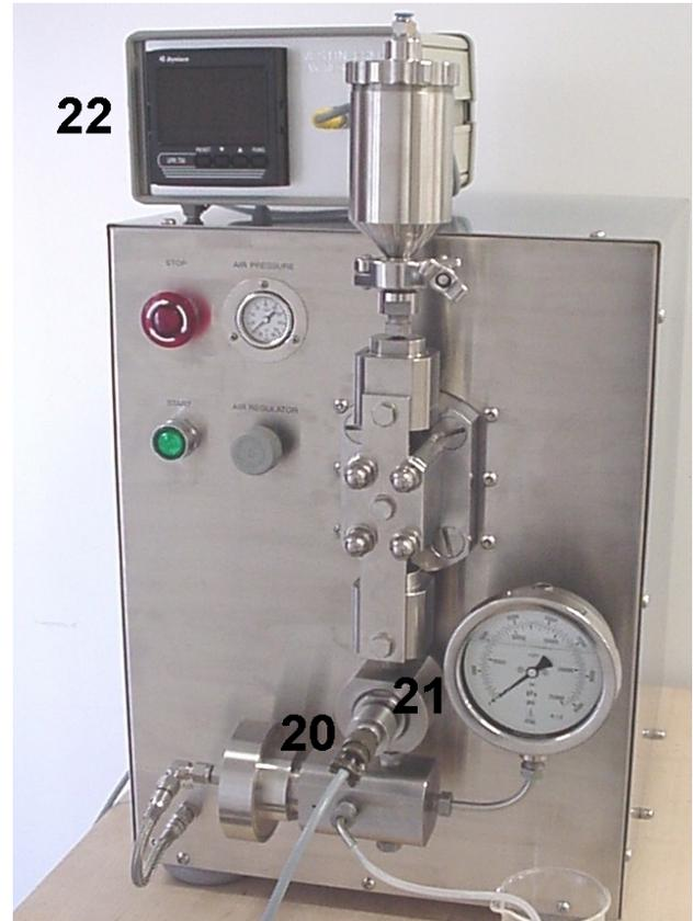
**Figure 6:** A flush diaphragm pressure transducer (20) in an adapter (21) attached to the digital peak reset meter (22).
