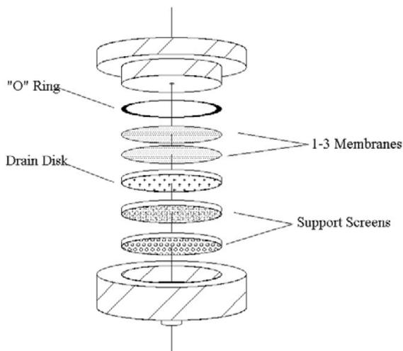
**Figure 3:** Filter/extruder assembly.
