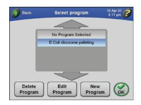
**NOTE** Pressing the **OK** button with a program name selected in this screen loads the program into the ultracentrifuge.
